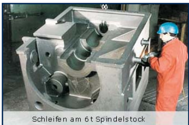
Schleifen am 6t Spindelstock
